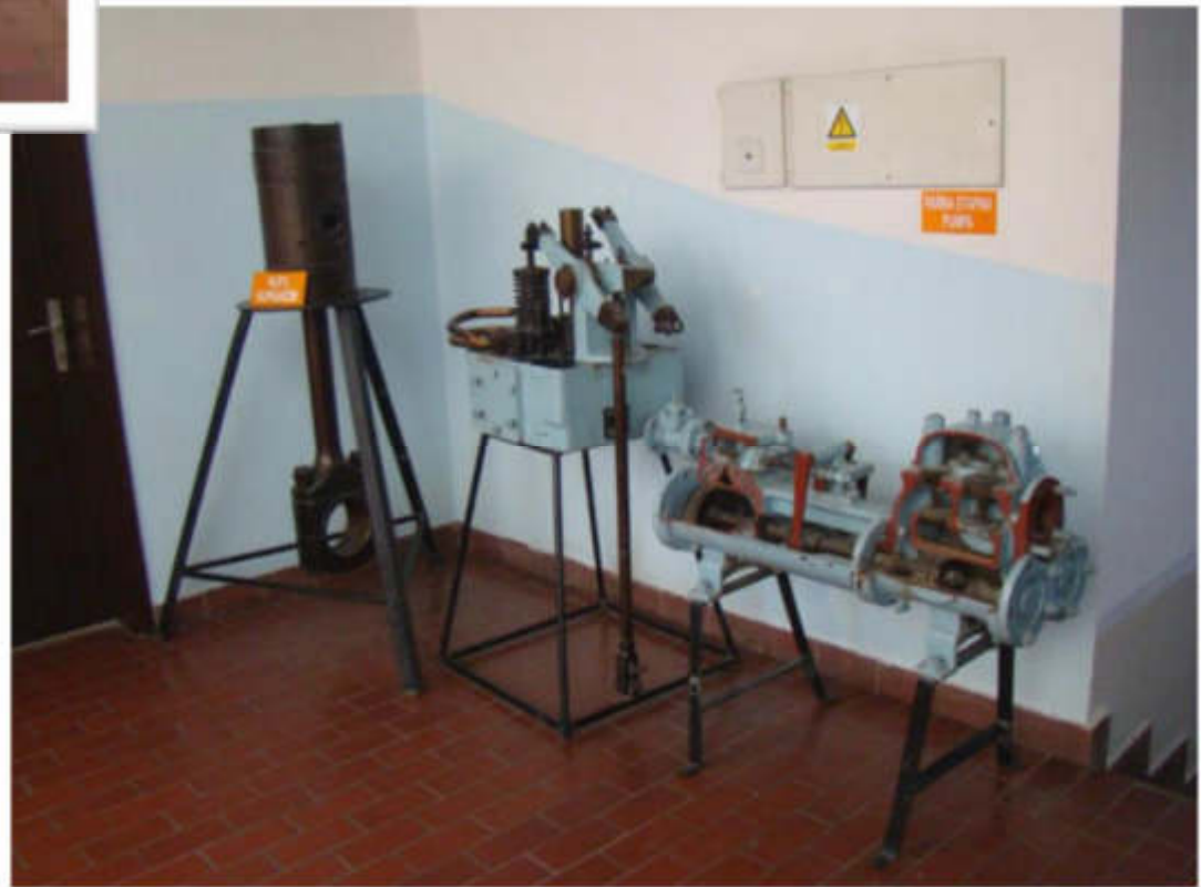
Part of the ship's engine; piston with a piston clip; steam pump
